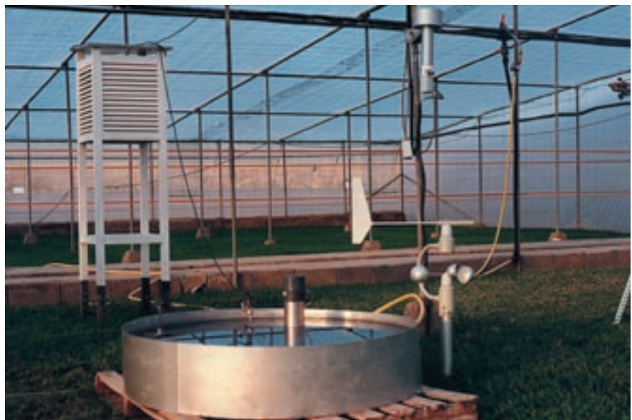
Evaporation pan (Class A) with an evapo- ration transmitter for measurement of evaporation, e. g. in the agricultural field
