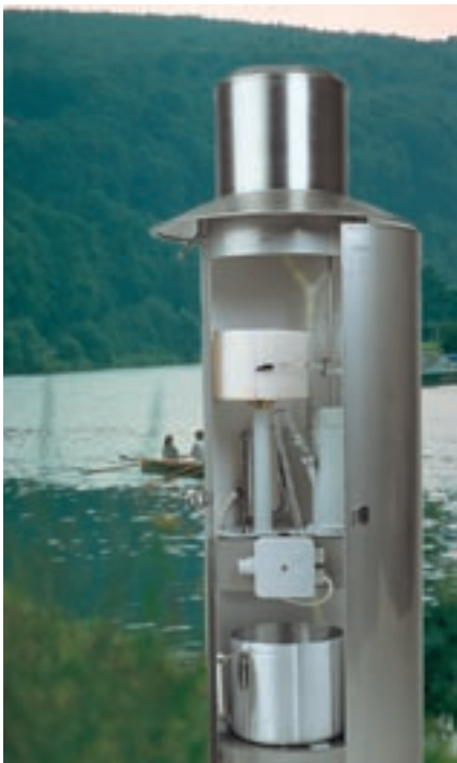
Precipitation meter for the mechanical acquisition of the precipitation for determining the water entry, e. g. in soil, artificial lakes, ponds etc.
